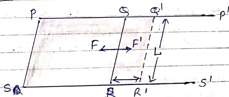
Consider a rectangular frame of wire  $P'PSS'$ . It is fitted with a movable arm  $QR$  as shown. This frame is dipped in a soap solution & then taken out. A film of soap solution will be formed within the boundaries  $PQRS$  of the frame.
