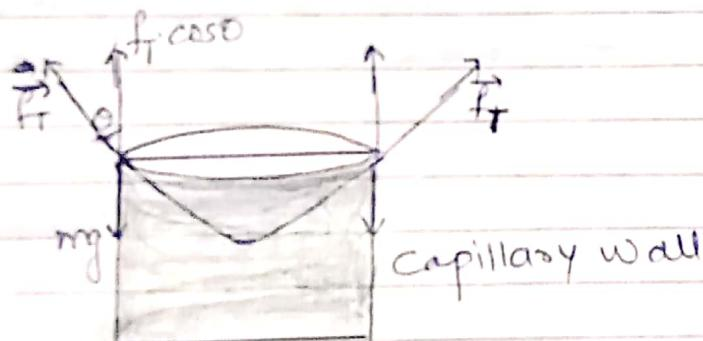
Consider a capillary tube dipped in a liquid which wets the walls of the tube. Therefore, angle of contact is acute & meniscus is concave.
