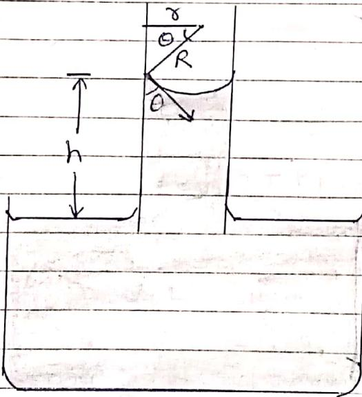
The pressure due to the liquid (water) column of height  $h$  must be equal to the pressure difference  $\frac{2T}{R}$  due to concavity.
