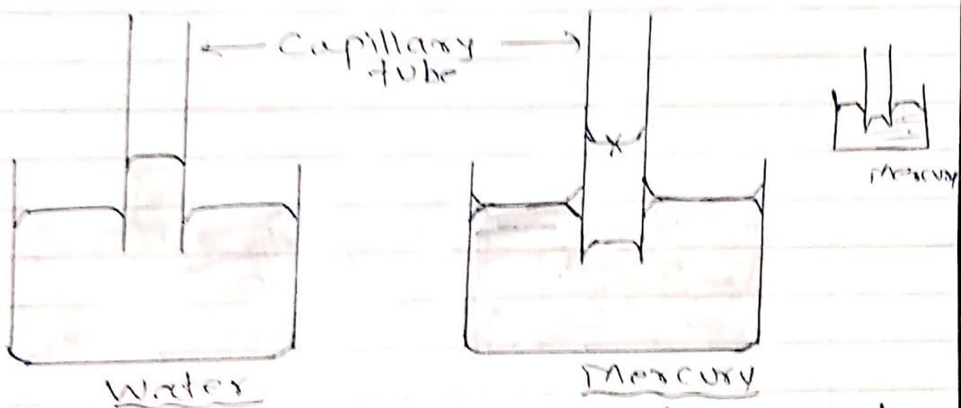
When Capillary tube is dipped in water which wets the capillary, the water level rises inside the capillary tube.
