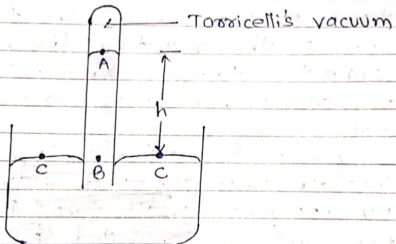
A glass tube 1m long & of diameter 1cm is filled with mercury upto its brim. It is then quickly inverted into a small dish containing mercury. As some mercury in the tube spills in the tube, a gap is created at the closed end of the tube.
