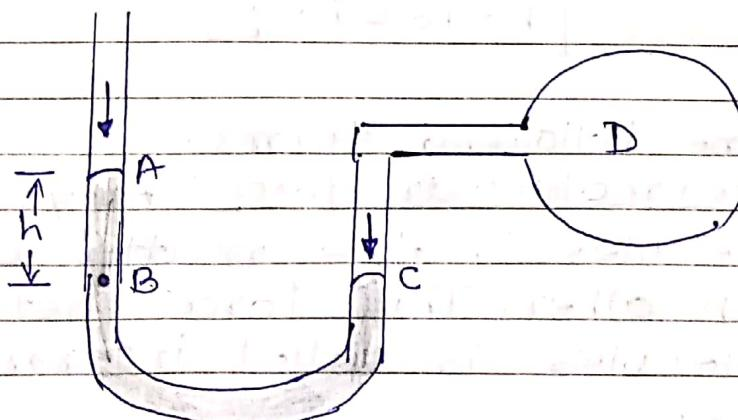
One arm of the manometer is open to the atmosphere & other is connected to the container 'D' of which the pressure  $P$  is to be measured.
