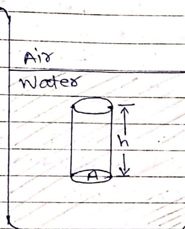
Consider a vessel filled with a liquid. Consider an imaginary cylinder of cross-sectional area  $A$  inside the container. Let the density of fluid be ' $\rho$ ' & ' $h$ ' be the height of the cylinder.
