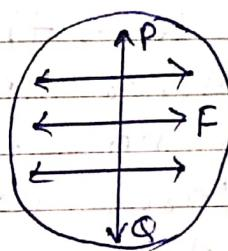
The free surface of a liquid in a container acts as a stretched membrane & all the molecules on the surface film experience a stretching force. Imagine a line  $PQ$  of length  $L$  drawn tangential to the free surface of the liquid as shown.
