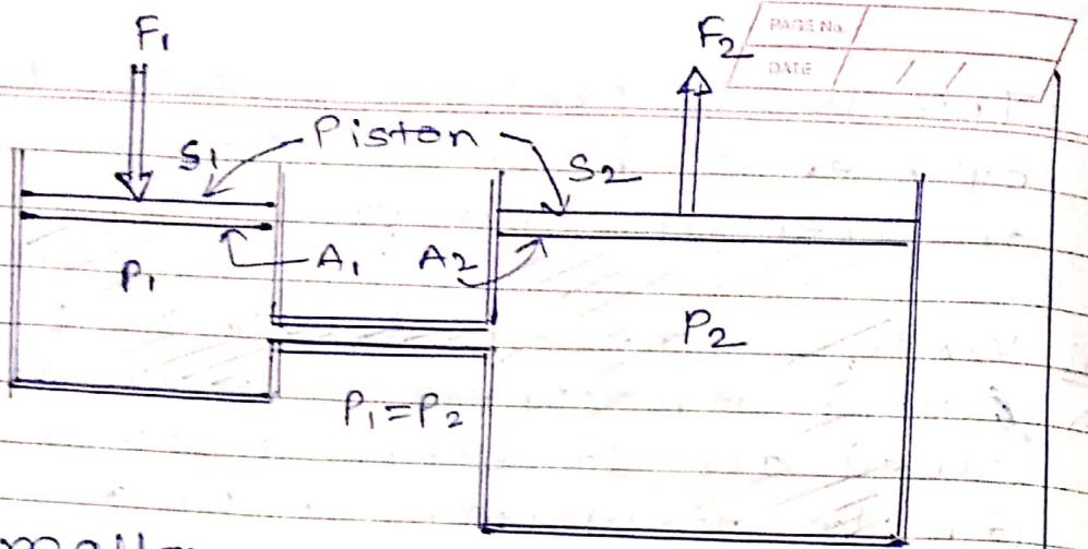
a smaller area of cross-section  $A_1$  while  $S_2$  has a much larger area of cross-section  $A_2$  ( $A_2 \gg A_1$ ).
